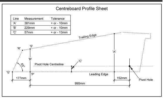
Measurements A, B and C are taken at 90° to the leading edge at the stated distance from the centre of the pivot hole. They shall be within the limits of measurement given on the Centreboard Profile Sheet.
