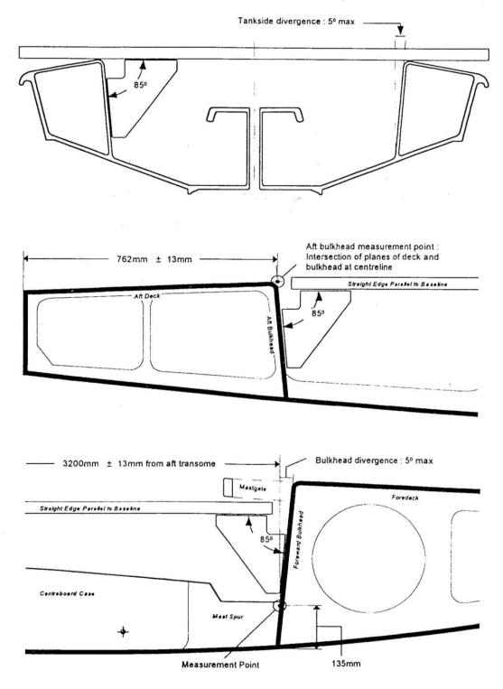
Measurement of position and angles of bulkheads and tanksides (ref : IFCR 9.7.1, 9.7.2, 9.7.4).
